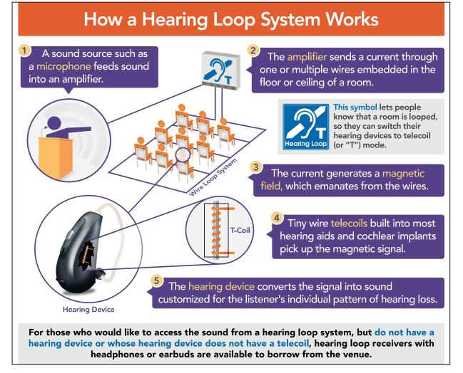
Hearing loop systems provide better communication access by transmitting sound directly to telecoil-equipped hearing aids, cochlear implants or other assistive listening devices. (Graphic courtesy of OTOjOY)
